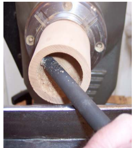
Hollowing the Red Birch box with the 3/8" handled tool.
