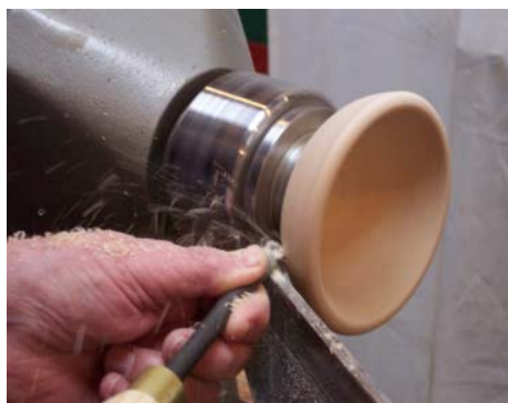
Turning the outside of the bowl with the 3/8" tool. The 1/2" was more stable for this operation.
