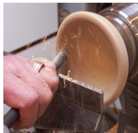
The 1/2" tool performed very well on the inside of the bowl. Creating fine shavings and cutting clean enough to be ready to sand.
