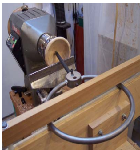
The 1/2" tool mounted in the Min-O-Bar from Turningways being used to hollow the bowl. I found it extremely easy to control the shape of the inside of the bowl with this set up.
